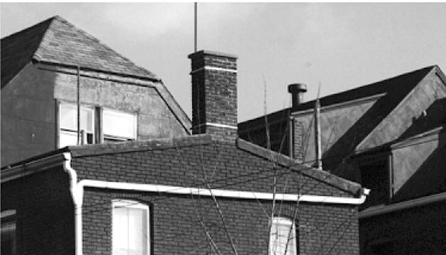
*Roofs with many intersecting ridges and valleys are prone to leaks. Regularly inspect the flashing to see that it is sound.*
